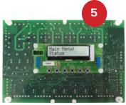
LCD mounted on back of MicroMag with new Standoffs
