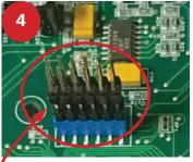
LCD Stacker Headers Pins on main board
